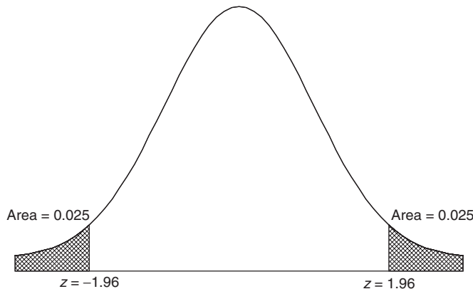
Fig. 17-3 Two-tailed test showing the critical region with \alpha = 0.05 .
